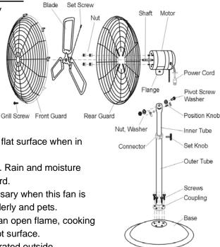
**WARNING:** be sure front and rear guard screws are completely screwed down in locking position before operation.
