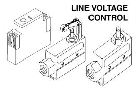
NOTE: If there are multiple manual doors on the opening, add plunger (part #9503SD020-P), or roller (part #9503SD020-RA) for each additional switch required.
