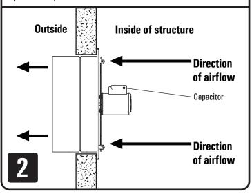
Using appropriate hardware (not provided) for your structure and the weight of your exhaust fan, secure the fan to your structure using the (4) pre-drilled holes on the mounting flange.
